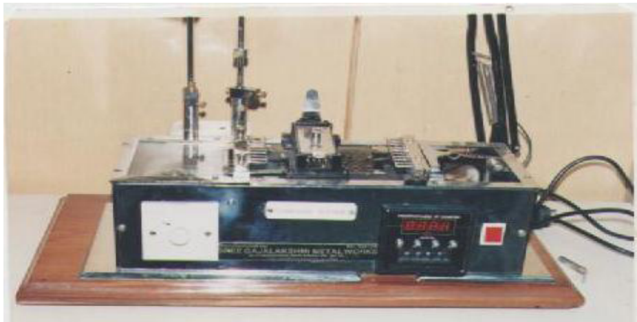
Figure 74: Duplon Cohesion Tester
